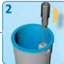
Lift float with cable to simulate fill
