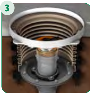
3 Replace Bellows, Reinstall Upper and Lower Rings
