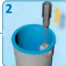
Lift float with cable to simulate fill
